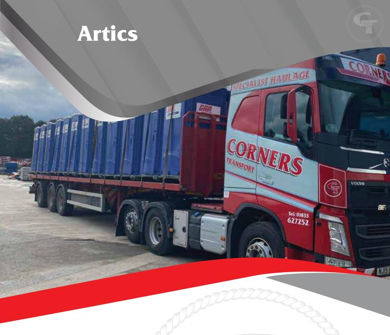
We operate number of tractor units from 44 ton to 80 ton carrying anything from steelwork too generators too static plant containers etc, all driver carry large number of straps chain etc so we prepared for any type of load. The trailer fleet we have stepframe plant trailers steering flats with post sockets and twist locks fully powered steered extenders up to 20m standard extenders and low loaders.
